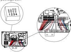
Fig 1.5 Inverter Box Wiring Diagram
