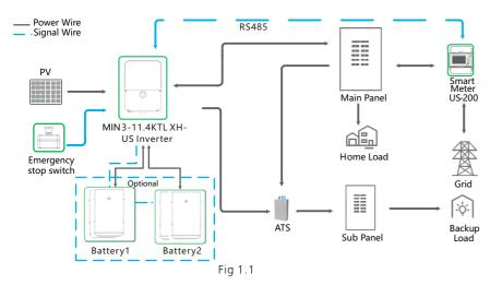
The system wiring diagram is as follows:
