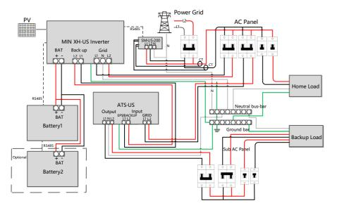
MIN 3K-11.4KTL-XH-US AC Couple system diagram is shown in the figure below:
